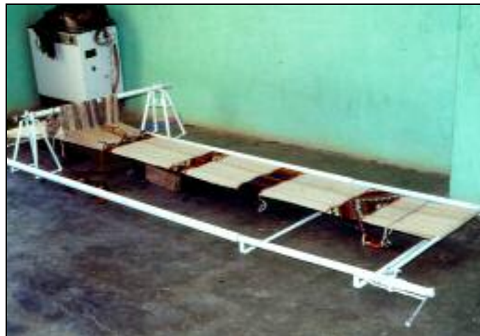
Fig. 12. A loom created for use by a settled Bedouin in Jordan, who works for Save the Children and makes small wool rugs of standardized patterns.
